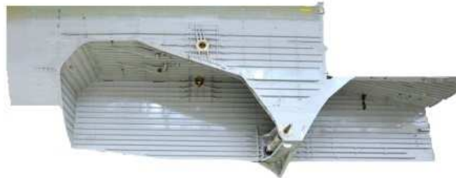
A380 Landing Gear Bay Section 15
