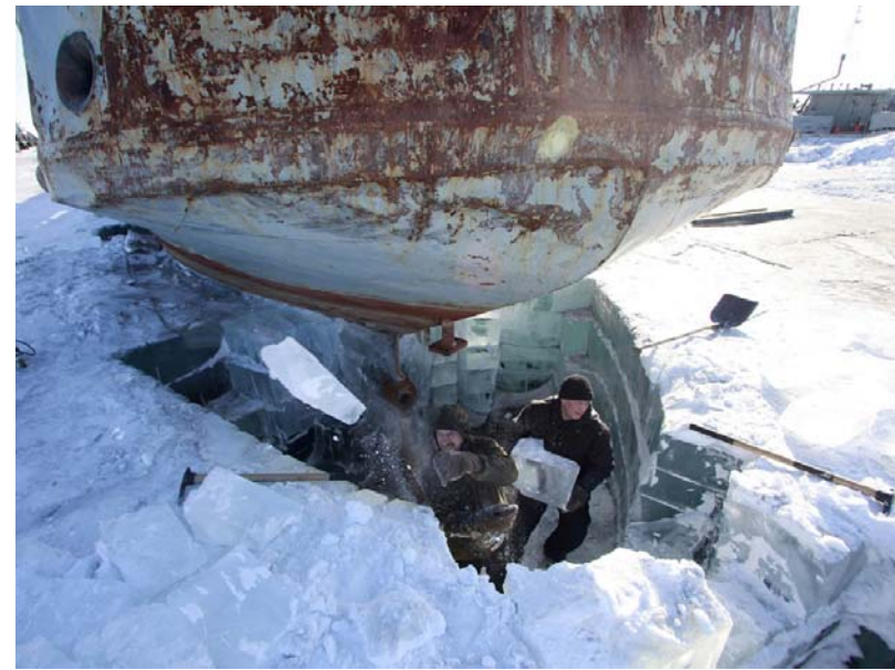
Workers remove ice blocks from under a vessel to release its propeller on the Khatanga River in Russia [ http://www.guardian.co.uk/world/picture/2010/apr/18/russia ]
