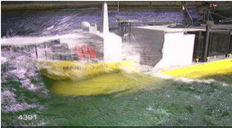
Picture 4: FPSO in 10,000yr Cyclonic waves
