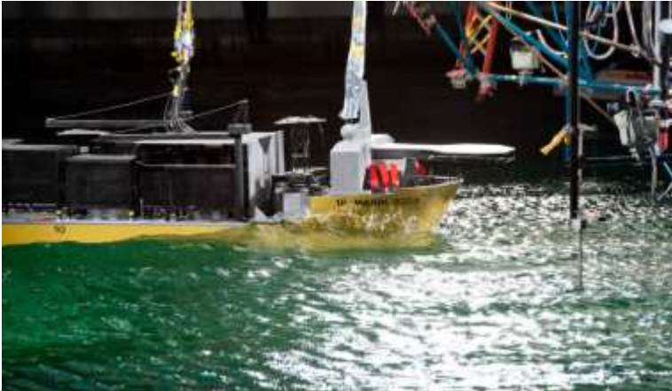
Picture 3: FPSO in 200yr Cyclonic waves
